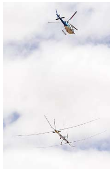
REPTeM helicopter borne system showing the new array.
